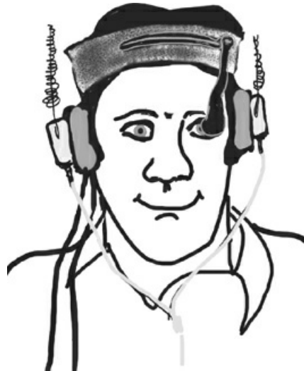
FIGURE 3-3 An eyeblink conditioning arrangement. The participant wears a headset that has a tube to direct a puff of air to the eye, a photocell to measure movement of the eyelid, and earphones for the presentation of auditory stimuli.
