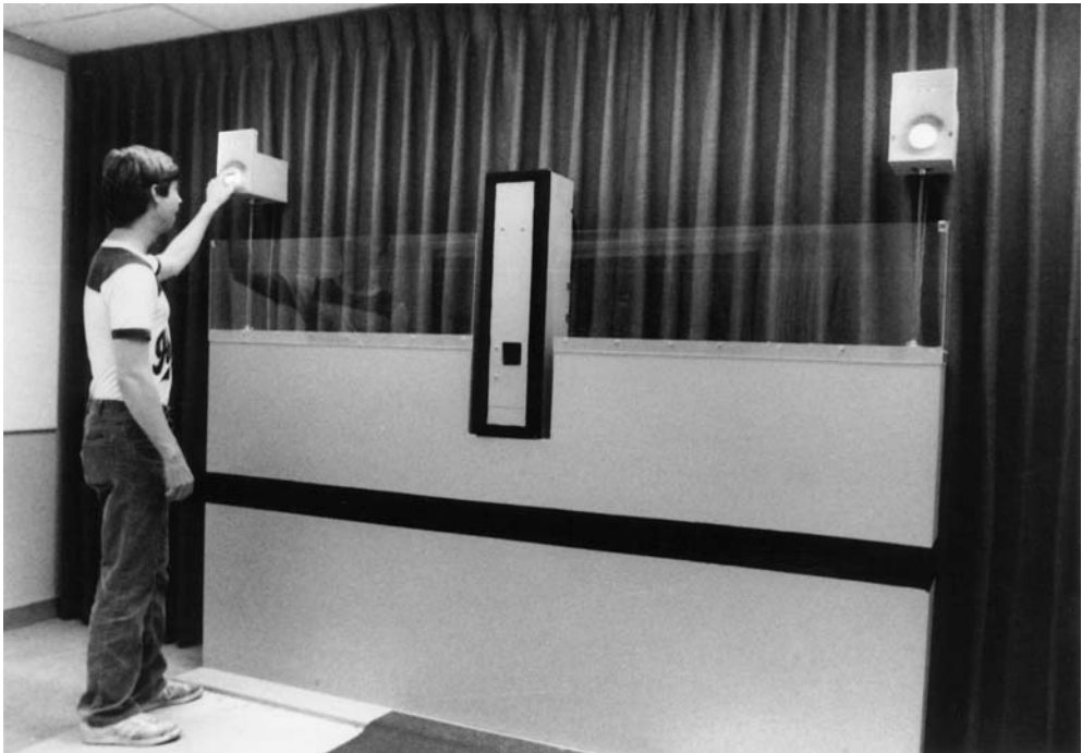
FIG. 9.2. A two-key operant chamber for humans. Pressing the keys results in money from a coin dispenser (middle), depending on the schedules of reinforcement. Author Photo.
